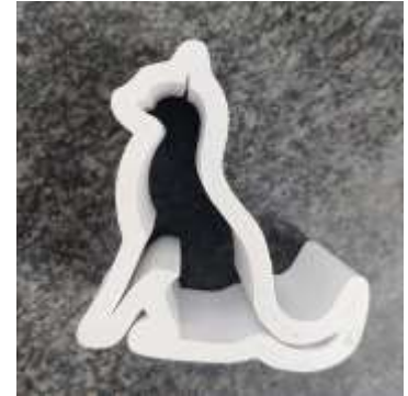
PLA/ABS PARTS PRINTED by FDM type 3D printer
