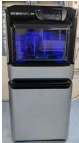
Stratasys J55 3D printer. Round Print Tray with up to 1,174cm 2 Print Height: 190mm
